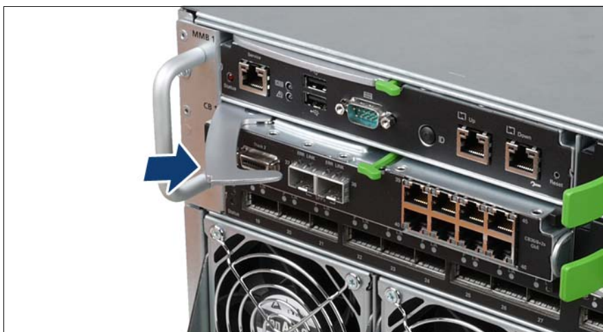
Figure 38: Locking the connection blade
